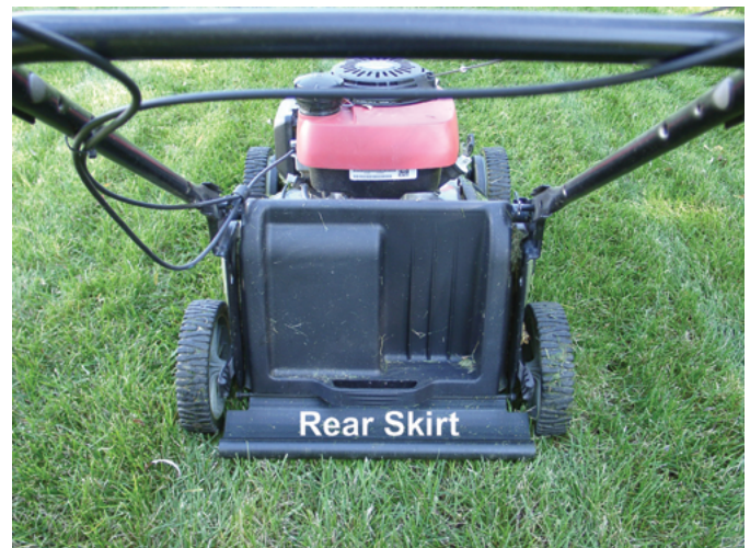
Figure 4. The rear skirt on rotary mowers can be used to create stripes.
